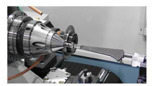
These parts are typically designed in Siemens NX, and ANCA provides a post-processor to create the necessary machine motions. After importing this file, ANCAam gives the operator the ability to manage specific process parameters, like speeds and feeds, offsets, and wheel selection, and dressing cycles. While ANCA's CIM3D package offers a full simulation to verify the grinding motion and to compare the expected part with the original model.
