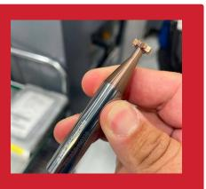
Moving on to hip stems, Gray said machining up and over these parts requires ball nose end mills in which the radius and its transition to the OD must be perfect. The end face gashing must also meet exactly at the center. "Any mismatch in the center of the ball nose will put a line in the hip stem, and that's not acceptable." Any error in the radius will create geometrical distortion in the part profile, he added. "We scan that whole radius to ensure it's correct."
