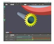
The GCX Linear software package includes multiple software components for manufacturing and resharpening pinion type gear cutters. It includes design, simulation, grinding sequence programming, wheel editing and wheel dressing, tool profile and spacing measurement, direct grinding path compensation supporting full virtualisation of the manufacturing process.
