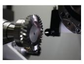
Due to the novelty of the skiving cutter, many industry benchmark GMMs (gear measurement machine) have yet to develop inbuilt mathematical models for evaluating the skiving cutter profile.
