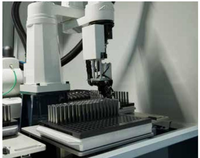
The CPX machine is offered with ANCA's own AR300 low cost loader for automated loading of tool blanks.
