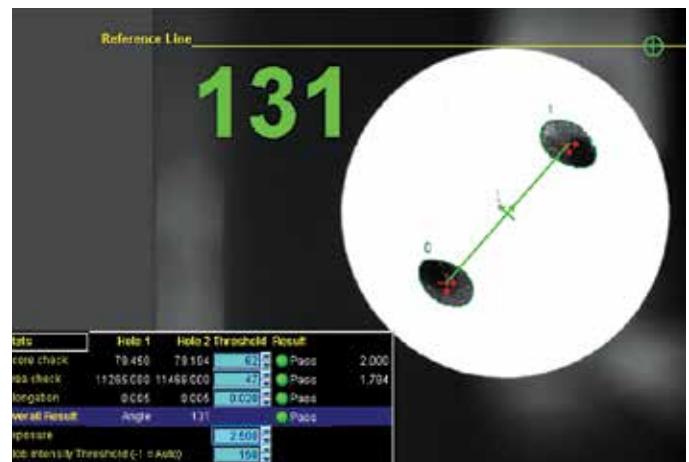
The tip of the tool appears white while the 2 coolant holes appear darker
