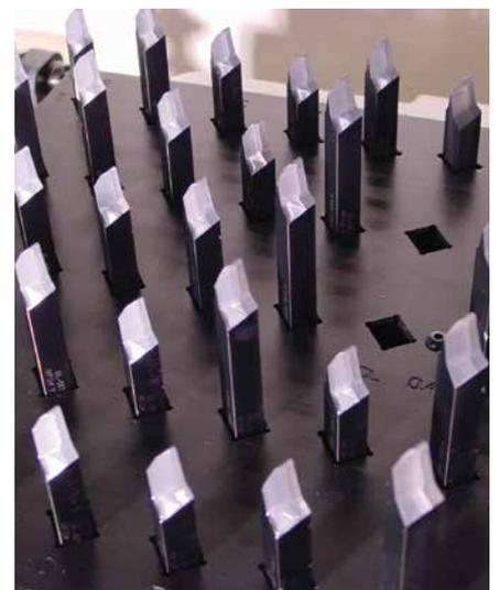
ANCA's RoboMate robot loader is a versatile and flexible automation solution. Using the accuracy and reliability of the Fanuc robot, RoboMate takes the tool directly from the pallet to the chuck in a single grip.
