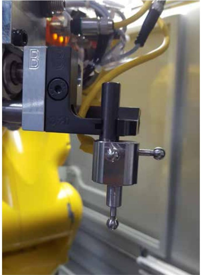
Contact touch probe held in the gripper
