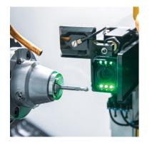
iView is a measuring system that is able to measure the ground tool while it is still in the work-holding on the machine. The image of the ground tool as taken by the iView camera is compared with an ideal overlay shape generated by the software. The tool size can then be compensated automatically based on the overlay.
