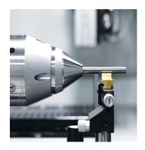
ANCA's Premierplus Collet Adaptors provides operators with a premium workholding range. The Premierplus Collet Adaptors use a new totally internal clamping mechanism. The spring pack in the adaptor provides the tool clamping force and prevents possible runout that was previously added if misalignment occurred between the drawbar and the collet. PremierPlus Collet Adaptors offer users the ability to make radial adjustments to the collet to obtain low run out on tools.
