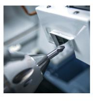
The LaserUltra system provides accurate and repeatable measurement of tools inside the machine. The LaserUltra can automatically measure OD, run-out, EOT, ball nose and corner radius profile tools. An air blast unit on the laser ensures that coolant or contaminants do not interfere with the measurement process.
