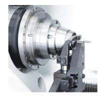
MicroPlus provides less than 3 micron tool runout. It is ANCA's #1 high accuracy work holding and tool support system. The MicroPlus system consists of the Flexi-Chuck assembly for workholding, and the Overhead Top Clamp Assembly (OTC) for too support. The Flexi-Chuck clamps and rotates the tool. The patented design allows the tool and the internal components to move independently of each other, minimising any misalignment.
