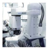
ANCA's designed and built low cost tool loader is fully contained within the machine canopy. The AR300 loader has 3 axes and is easily set up and controlled via the touch screen and remote handheld pendant. It provides customers with an affordable automatic tool loading solution and is perfect for low-volume production runs.
