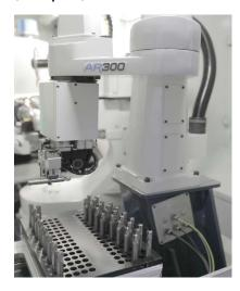
ANCA's designed and built low cost tool loader is fully contained within the machine canopy. The AR300 loader has 3 axes and is easily set up and controlled via the touch screen and remote handheld pendant. It provides customers with an affordable automatic tool loading solution and is perfect for low-volume production runs.
