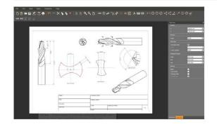
ToolDraft is used for creating 2D cutting tool drawings from a simulated tool or direct from ToolRoom. This is built on the foundation of CIM3D engine projecting a 3D model into accurate 2D projection views. This will help customers to create drawings of cutting tools manufactured on ANCA machines without relying on third party software.
