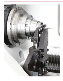
MicroPlus provides less than 3 micron tool runout. It is ANCA's #1 high accuracy work holding and tool support system. The MicroPlus system consists of the Flexi-Chuck assembly for workholding, and the Overhead Top Clamp Assembly (OTC) for tool support. The Flexi-Chuck clamps and rotates the tool. The patented design allows the tool and the internal components to move independently of each other, minimising any misalignment.
