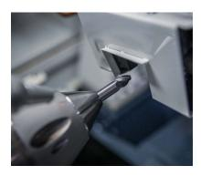
The LaserUltra system provides accurate and repeatable measurement of tools inside the machine. The LaserUltra can automatically measure OD, run-out, EOT, ball nose and corner radius profile tools. An air blast unit on the laser ensures that coolant or contaminants do not interfere with the measurement process.
