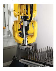
The Fanuc Robot Loader is a versatile automation solution that is located completely within the FX Linear machine. It provides automatic tool loading, enabling extended periods of unmanned operation, for maximised productivity.
