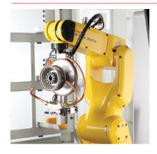
Used in conjunction with the Robot Loader. 6 wheel packs and coolant manifolds are loaded together, stored on a frame next to the robot. A docking station allows the wheel pack to be located close to the wheel spindle for fast wheel change cycle times. The wheel changer is totally contained within the FX7 canopy.
