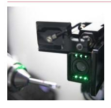
iView is a measuring system that is able to measure the ground tool while it is still in the work-holding on the machine. The image of the ground tool as taken by the iView camera is compared with an ideal overlay shape generated by the software. The tool size can then be compensated automatically based on the overlay.
