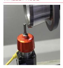
The auto wheel pack qualification probe is used to accurately measure grinding wheels inside the machine. The Wheel Probe uses a Renishaw probe to qualify the wheel pack. It is possible to measure the front surface location, back surface location, wheel diameter and toroid radius of a grinding wheel. It eliminates the need for operator intervention which ensures consistent measurement results.
