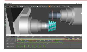
CIMulator3D simulates the programmed tool path exactly as it would be ground on the machine. New tool programs can be verified for size, shape, machine clearance and even cycle time estimates. CIMulator3D maintains continuous work flow through the machine by reducing development time and trial grinding.
