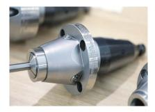
ANCA's Premierplus Collet Adaptors provides operators with a premium workholding range. The Premierplus Collet Adaptors use a new totally internal clamping mechanism. The spring pack in the adaptor provides the tool clamping force and prevents possible runout that was previously added if misalignment occurred between the drawbar and the collet. PremierPlus Collet Adaptors offer users the ability to make radial adjustments to q the collet to obtain low run out on tools.
